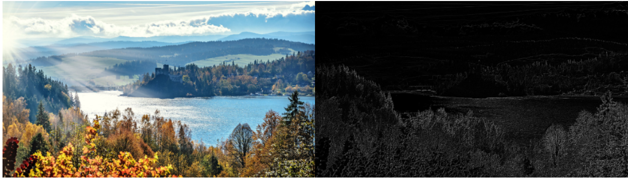
Figure 5.3 Example of input and output image from the Sobel core
